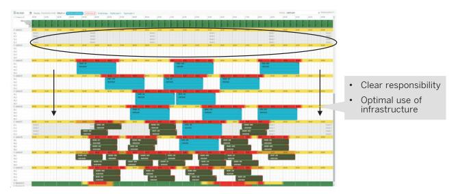
In the first half of the example, responsibility is clear (i.e. different handlers are allocated to different resources), but the use of infrastructure is suboptimal. Using common areas (second screenshot) by allocating the same lateral to several handlers throughout the day leads to an optimal use of infrastructure (i.e. in the example the two top laterals can be freed up across the full day) without sacrificing clarity
